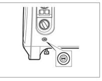
Fig. 26a. Trunk lid latch actuator switch (in the design variant)
