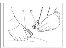
Fig. 14a. Fastening the seat belt
