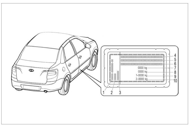
Fig. 68. Passport details. Installation site of name plate - center pillar, RH
