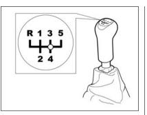
Fig. 37a. Gear change lever in mechanical transmission
