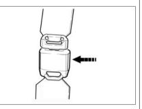
Fig. 14c. Mini-lock of the back middle seat passenger seat belt
