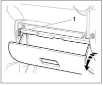
Fig. 41c. USB connector location
