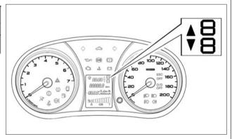
Fig. 30. Gearshift prompter function in instrument panel
