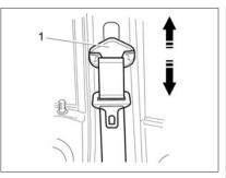
Fig. 14b. Adjusting the seat belt (in the design variant)
