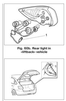
Fig. 60c. Shelf support clip removal
