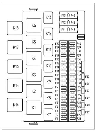
Fig. 58. Fuse block and relay of passenger compartment
