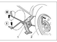
Fig. 54. Lifting the vehicle when replacing the wheels
