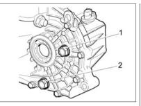
Fig. 46b. Gearbox oil level checking (in the design variant)
