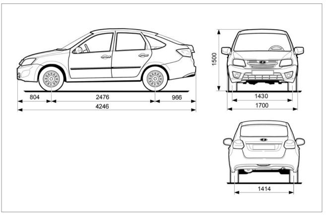
Fig. 67. Overall (reference) dimensions of the vehicle 2191 «liftback»
