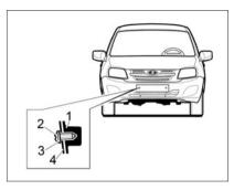
Fig. 42a. Fastening of number plates
