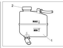
Fig. 49. Expansion chamber
