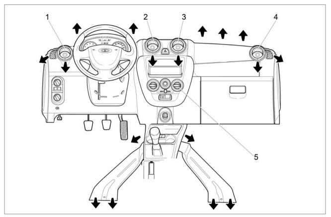
Fig. 39. The directions of the air flows out of deflectors and ducts
