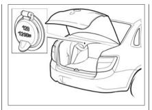
Fig. 21d. Socket for additional electrical equipment in luggage compartment (for some vehicles)
