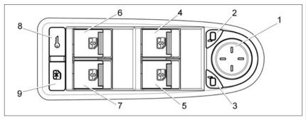
Fig. 6b. Driver's door module (in the design variant)
