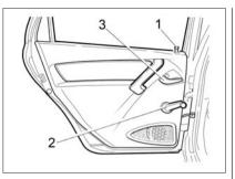
Fig. 7b. Rear door with the speaker (in the design variant)
