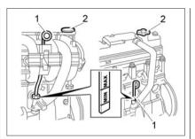
Fig. 45. Engine case oil level checking
