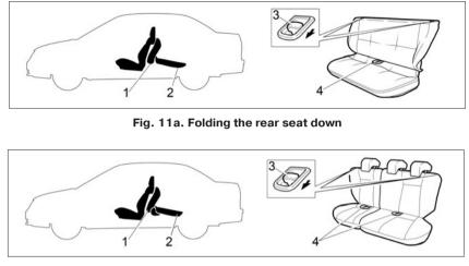
Fig. 11b. Folding down the rear seat with the headrests (in the design variant)
