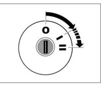
Fig. 36. Ignition starter switch
