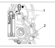
Fig. 46a. Gearbox oil level checking
