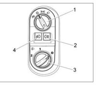
Fig. 32a. Lighting engineering control module and dipped beam adjuster
