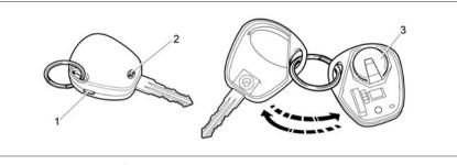
Fig. 56. The remote control battery replacement
