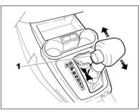
Fig. 37c. Gear change lever in automatic transmission
