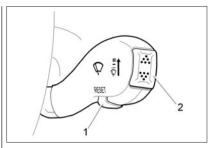
Fig. 31. Trip computer control buttons on the wiper lever (in the design variant)
